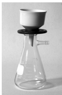
Büchner flask (Filter flask) Büchner shown with funnel and universal rubber filter adapter
