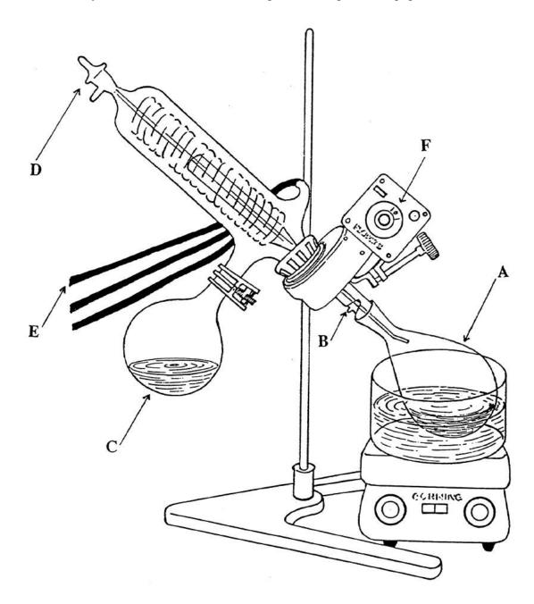
**Figure 5.1.** A Büchi Rotavapor (Model used may not be exactly as illustrated.)
