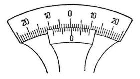
Figure 7.5. Reading the Vernier scale on the polarimeter
