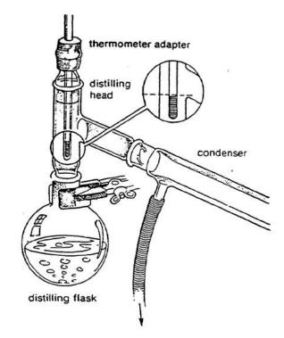
Figure 3.3. Thermometer placement during a simple distillation
